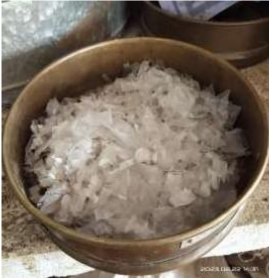
Figure 3.2 Plastic waste strips
