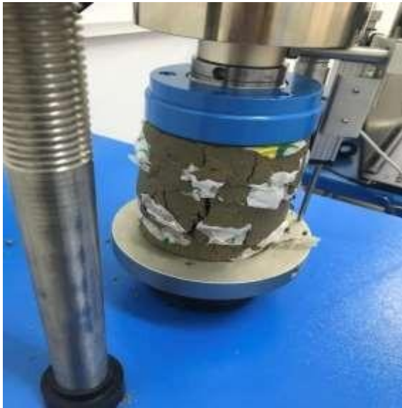
Figure4.13:UCS result showing the failure under stressfor0.2%plasticcontent
