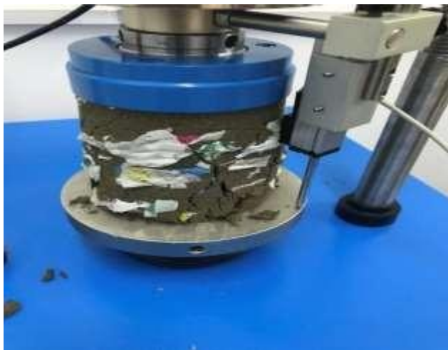
Figure4.15:UCS result showing the failure under stressfor0.4%plasticcontent
